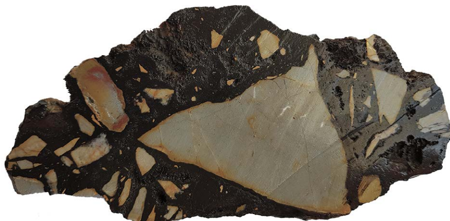
Figure 3: Picture of breccia sample collected from the Khao Soon Tungsten Project. The black material is fine grained wolframite (tungsten trioxide). Spot hhXRF analysis ranges from 21-43% WO 3 . Scale approximately 60% original sample.
